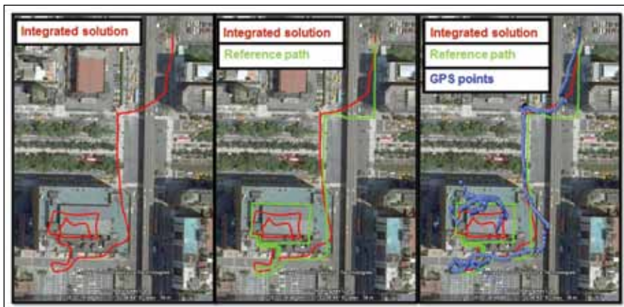
FIGURE 6 Comparison of GPS-only (blue) and integrated (red) positioning solutions, with reference truth (green) path in downtown Taipei
